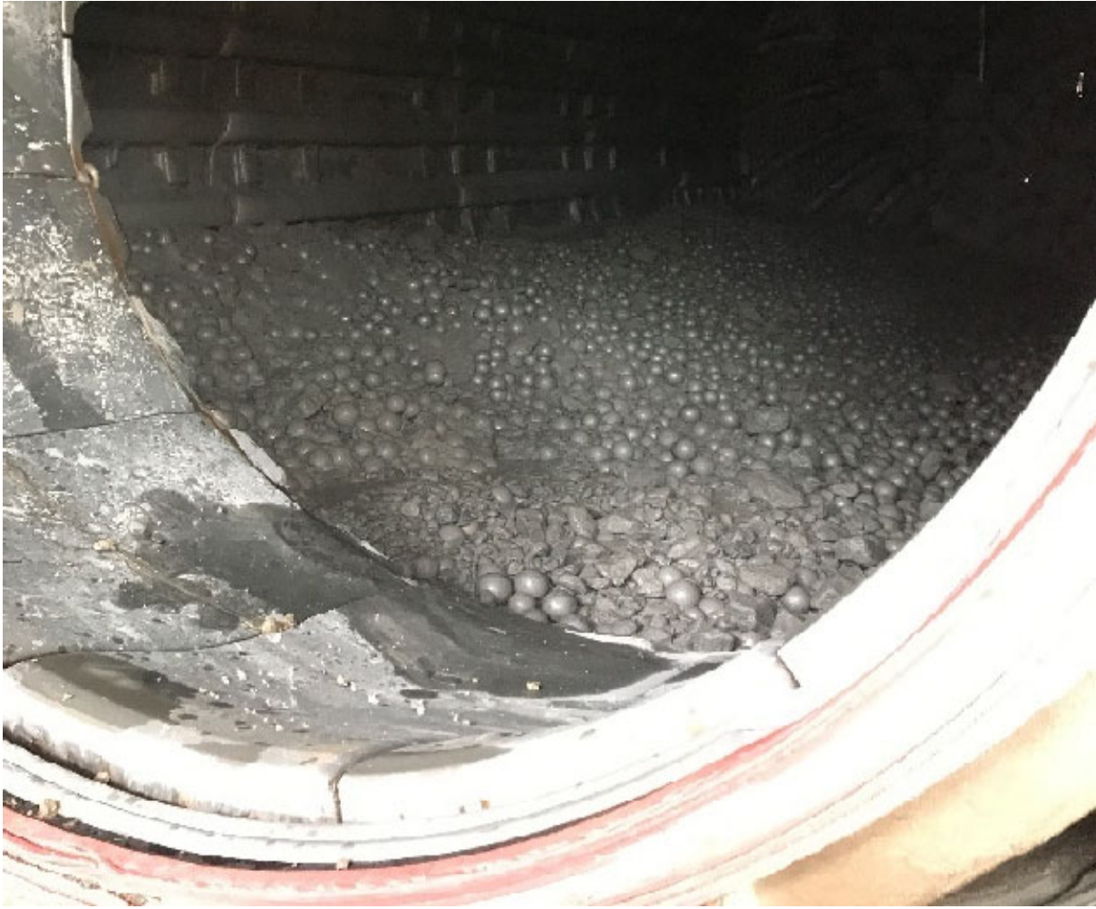
Figure 1—SAG mill crash stop charge
