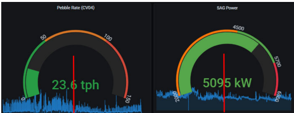
Figure 10—Scats and power with improved density stability, before and after control mod
